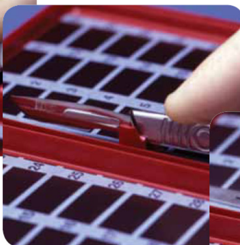
Step 2: Slide forward until blade "catches".
